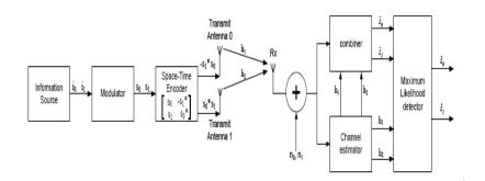
Figure 2: A Block diagram of alamauti's STBC
